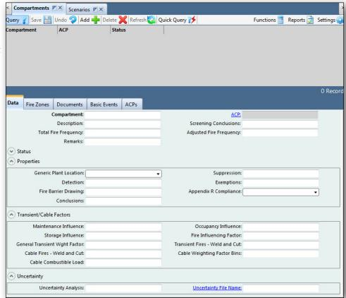
a fire zone location. Based on the permit's status, SAFE automatically adds transient combustibles to or removes them from a fire zone and updates the fire zone's combustible loading calculations. The fire protection combustible loading feature also calculates fire severity. SAFE fire area records track fire zone specific data for suppression, detection, and exemptions.
